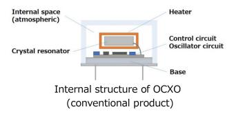
In general, OCXOs achieve a high level of stability by maintaining the temperature of its crystal oscillator constant to minimize the effects of the temperature characteristics. Conventional OCXOs have a large core, which is an oscillator circuit containing a crystal oscillator, with the corresponding amount of heat capacity and heat dissipation, consuming a significant amount of power consumption. In addition, conventional OCXOs are
